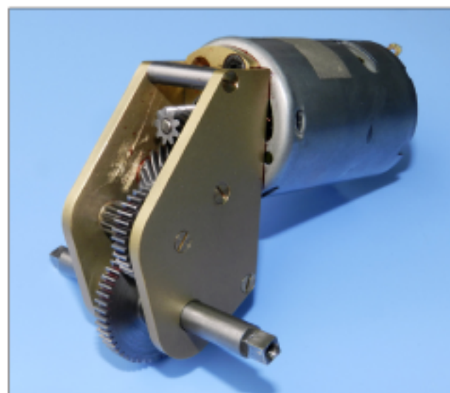
(Above) GBG3 30:1 gear ratio; fitted with a 36x50 Mabuchi 24volt motor.
